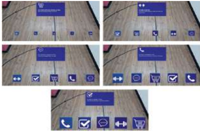
Fig. 1. AR scene with buttons of different sizes: 15, 25, 35, 45, and 55 mm at the distance of 450 mm.
