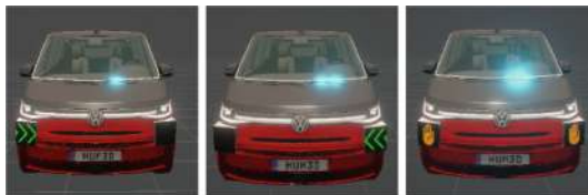
Fig. 1. Illustration of the eHMI concept when the AV: a) brakes for the AV side; b) brakes for the opposite side; c) drives through.
